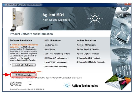
c. Select the option 'U1084A Installation', which will install the software required for your U10xxA series product, without the Agilent IO Libraries Suite which is not required for these products.
